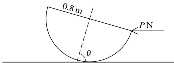
A uniform solid hemisphere of weight 60 N and radius 0.8 m rests in limiting equilibrium with its curved surface on a rough horizontal plane. The axis of symmetry of the hemisphere is inclined at an angle of  $\theta$  to the horizontal, where  $\cos \theta = 0.28$ . Equilibrium is maintained by a horizontal force of magnitude  $P$  N applied to the lowest point of the circular rim of the hemisphere (see diagram).
