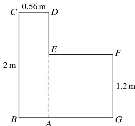
A uniform lamina is made by joining a rectangle  $ABCD$ , in which  $AB = CD = 0.56 \text{ m}$  and  $BC = AD = 2 \text{ m}$ , and a square  $EFGA$  of side  $1.2 \text{ m}$ . The vertex  $E$  of the square lies on the edge  $AD$  of the rectangle (see diagram). The centre of mass of the lamina is a distance  $h \text{ m}$  from  $BC$  and a distance  $v \text{ m}$  from  $BAG$ .
